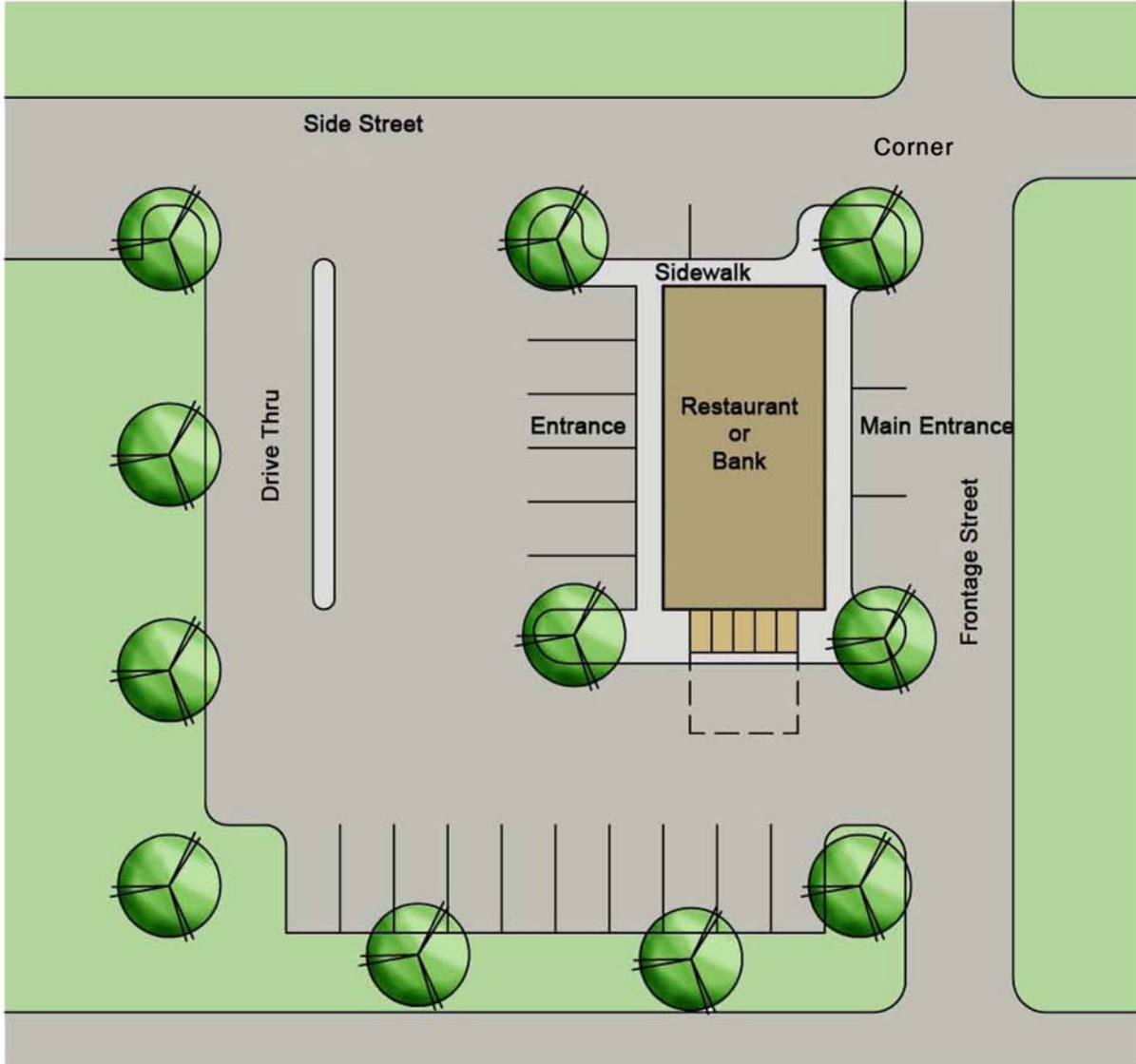
Lot Diagram: Drive-thru Restaurant, Take-home food shop, or Bank on a Corner (Building “Anchors” Corner)
